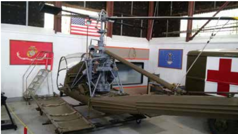
Above: Bob Crapser installed stretchers on the Hiller OH-23A (photo by Kevin Drewelow)
